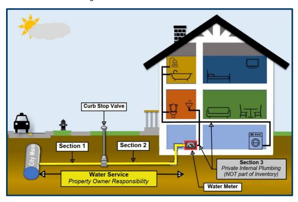
As part of the water service line inventory, City staff and consultants used a variety of methods to determine the material of Section 1 and Section 2 of your water service in the diagram above. It is important to note that Section 3, which is the internal plumbing of your home after the water meter, was not part of the inventory efforts mandated by the EPA and MDH. All three sections of the water service are owned by the private property owner in the City of Hastings.
