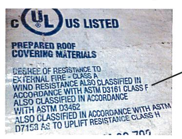
As long as the wind resistance is a Class D, F, G or H or reads 90 MPH or higher than the shingles are code acceptable for wind.
