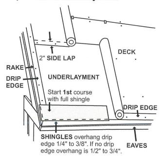
Installation: When applying underlayment, keep the product as wrinkle-free as possible. Unroll the underlayment parallel with the eaves. The underlayment should go over eaves' drip edge flashing, but go under the rake's drip edge flashing.
